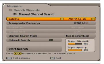
Use the buttons to select the satellite on which the transponder you wish to scan is located. Make sure your reception system is aligned to the selected satellite. You can search only one transponder at a time. If you wish to search several transponders on a satellite, you should start an automatic search of the
